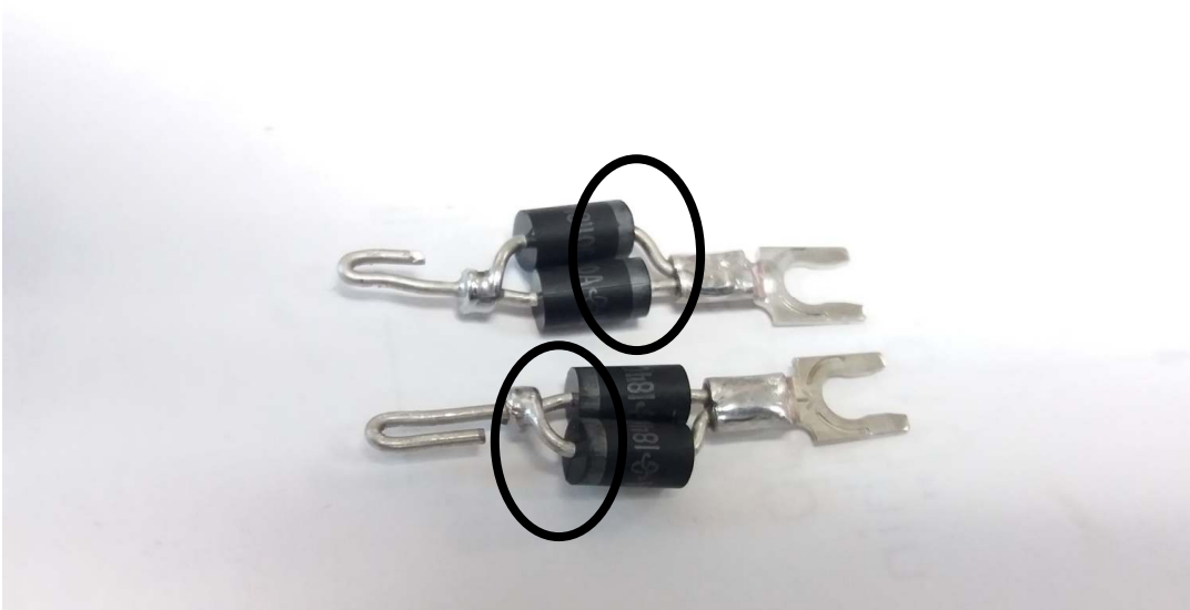
Fig 1. Pair of Diodes. Notice the orientation (polarity) of the stripe. (both are different)
