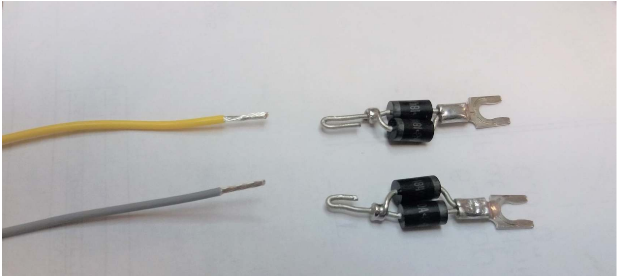
Fig 3. Terminals cut off and wires stripped.
