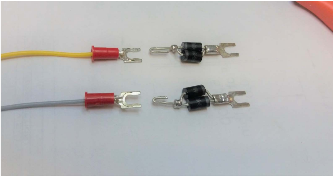
Fig 2. Shows + and - 15 V power terminals disconnected from power supply (+15 YELLOW and -15 GRAY)
